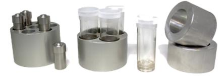
A range of vial adapters are available to run multiple smaller vials in the Mixer/Mill clamp. Up to seven small vials may be run simultaneously in each clamp.
