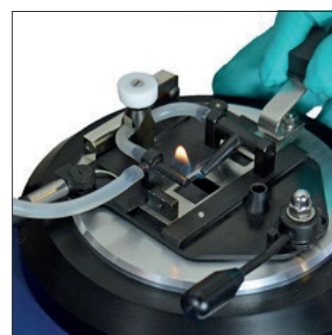
Dip the test flame, flash detection is automatic
