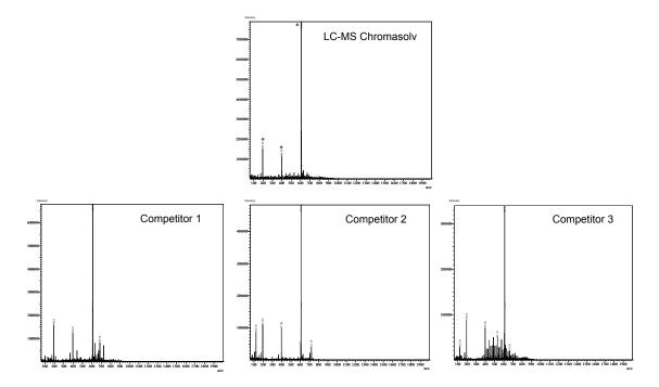
The quality and purity of Acetonitrile Chromasolv LC-MS (34967) was evaluated against the comparable solvent from three leading global laboratory chemical suppliers using LC-MS. The ESI+-mass spectra shows that Chromasolv LC-MS acetontrile has a much better impurity profile than competitive products.
