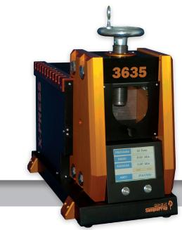
Ideal for repetitive pressing of sample pellets for XRF, IR and other analytical techniques. Typical samples include: Cements, Rocks, Minerals, Soils, Ceramics, and Pharmaceuticals.
