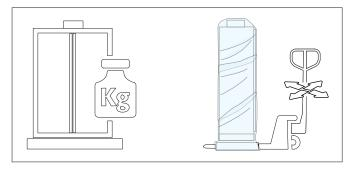
Use a pallet truck to move the cabinet, which must be placed vertically and be secured and protected against slipping up to its final installation site.
