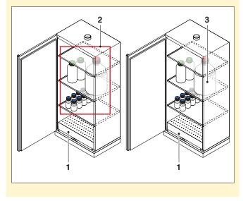
Use of the support surface of the collection tray (1) is only allowed in combination with a perforated sheet metal element.
